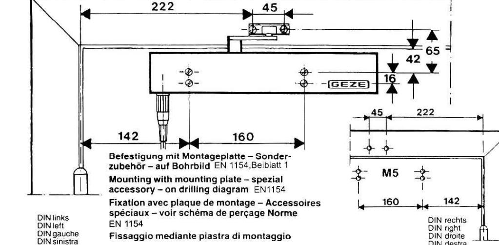
Fasten closer in accordance with drilling template.
